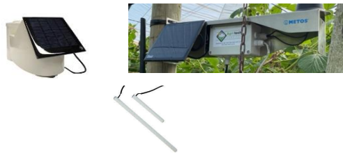
Moisture, EC and temp from the probes
