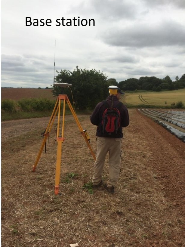
Setting up RTK Base Station
